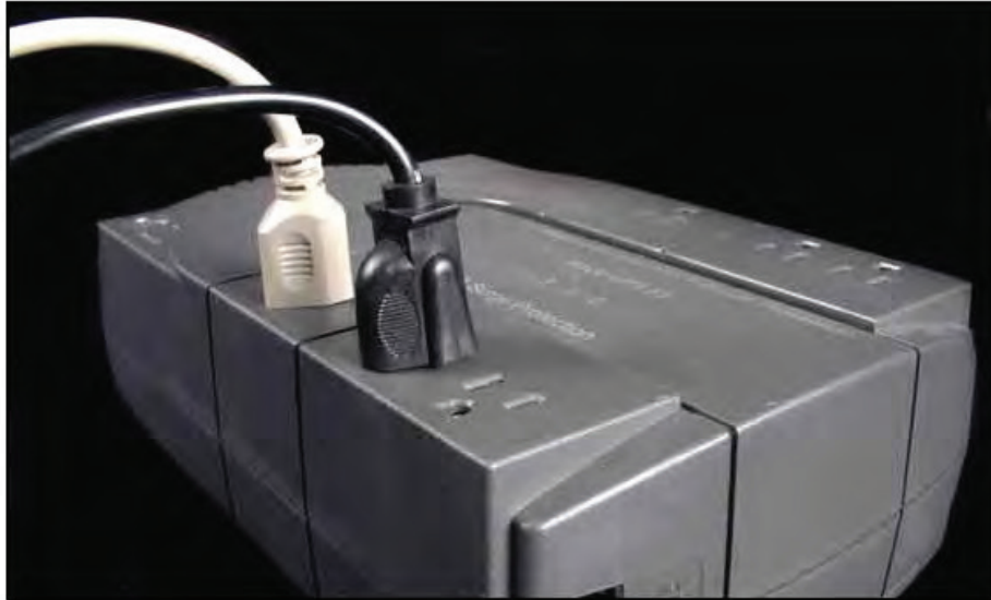
Figure 8-4: Power connectors connected to a UPS.
