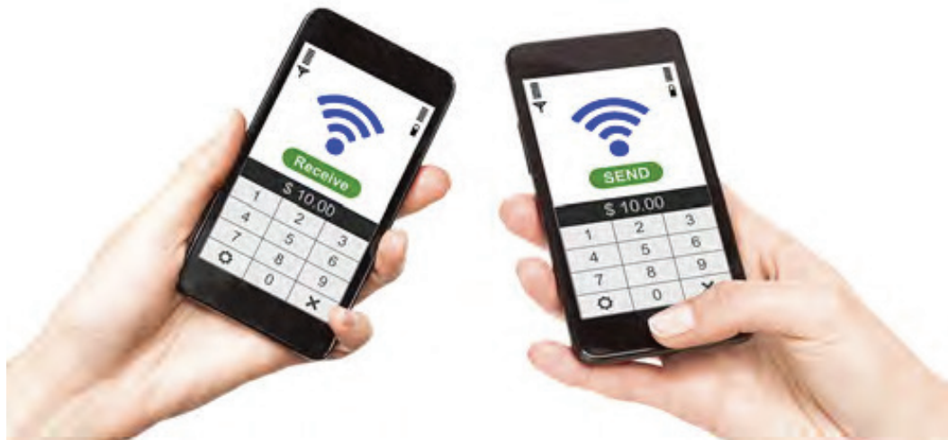
Figure 6-2: NFC allows for data exchange between two devices that are within inches of each other.
